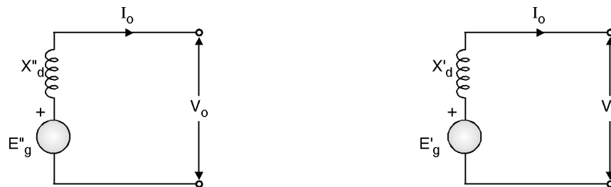
(a) Model for analysis of subtransient current (b) Model for analysis of transient current Fig. 1.5.2
