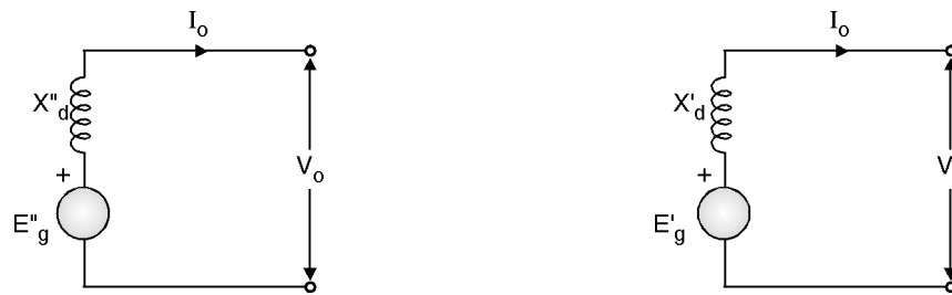
(a) Model for analysis of subtransient current (b) Model for analysis of transient current Fig. 1.5.2
